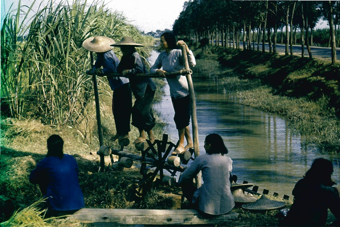
ABOVE (33) A treddle-operated square-pallet chain pump being used in contemporary China for raising water for irrigation.
