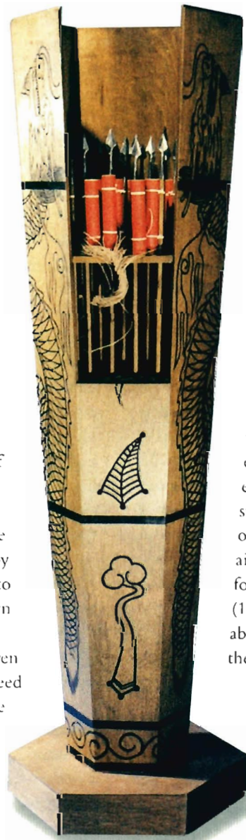
LEFT (178) A reconstruction, from a medieval drawing and textual descriptions, of a fourteenth-century 'bees' nest' rocket-launcher. The rockets are strapped near the tips of the arrows.
