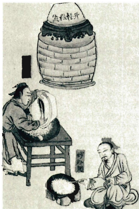
LEFT (93) A painting from Essentials of the Pharmacopoeia Ranked According to Nature and Efficacy: Imperially Commissioned , of the year 1505, edited by Liu Wen-T'ai for private deposit in the Imperial Library and not intended for publication. We see here the process of sublimation of calomel (mercurous chloride). The figure on the left gently brushes the crystals from the sublimation lid with a feather. This same process was used for collection of pure crystals of human sex and pituitary hormones from human urine by the second century BC. From 150 gallons of human urine, 2 to 3 ounces of hormone crystals could be produced by this method. (Biblioteca Nazionale Centrale Vittorio Emanuele II, Rome.)
